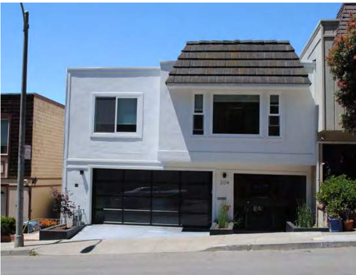
[5-23] 304 Gold Mine Drive | This Galli house recently underwent a major remodel. Although the distinctive Neo-Mansard roof is retained, almost all other features have been lost. While the windows are in roughly the same layout, the large white vinyl frames and sash windows are not compatible replacements. [Hannah Simonson]
